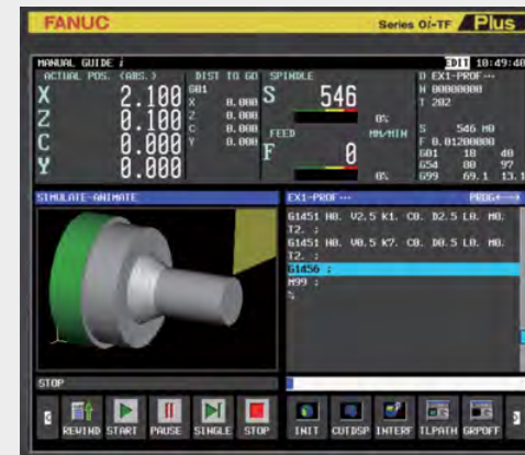
Check cutting result using cutting simulation
