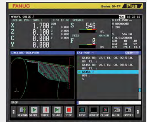
Check cutting path using cutting simulation
